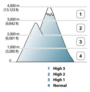
You can set the altitude value from **Device Settings** in Samsung Easy Printer Manager program or **Machine** section in Printer Settings Utility program.
